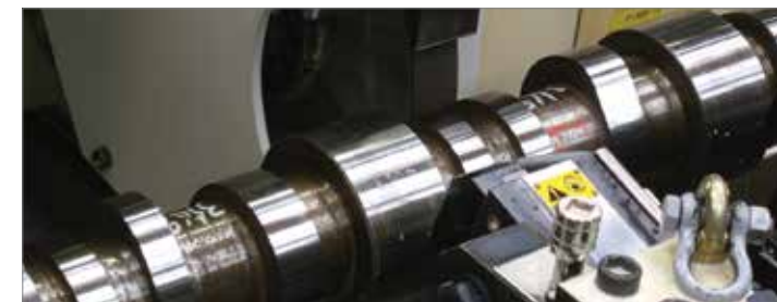
Finish grinding intake, exhaust cam lobes and injectors
