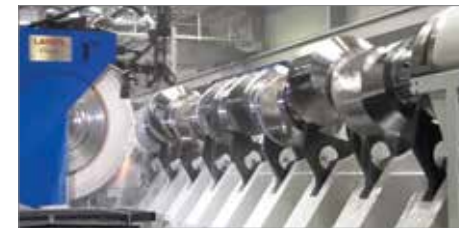
Grinding of pins on 6,500 mm crankshaft
